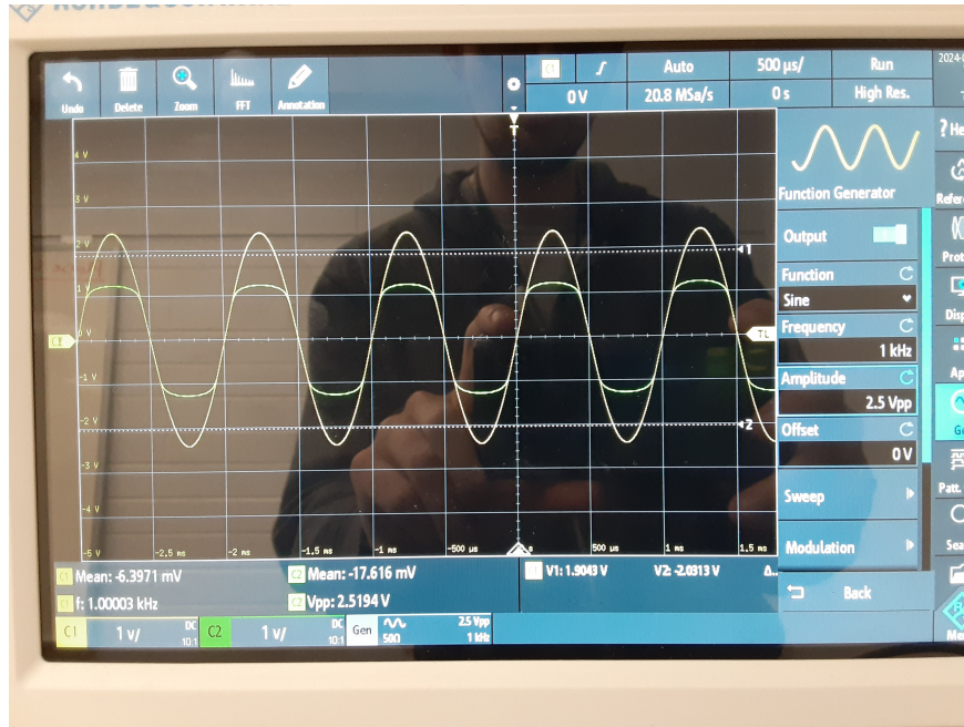
Figure 10. Behaviour of the circuit from Prelab Exercise 11 given a 5 V peak-to-peak sinusoidal input. v_{in} is yellow and v_{out} is green.
