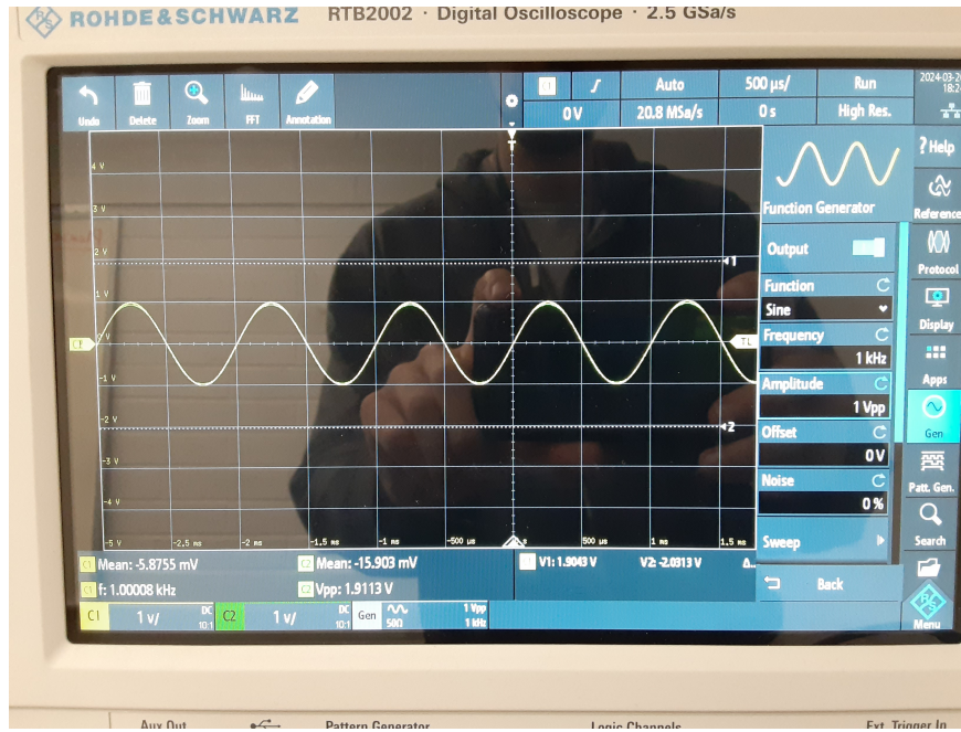
Figure 9. Behaviour of the circuit from Prelab Exercise 11 given a 2 V peak-to-peak sinusoidal input. v_{in} is yellow and v_{out} is green, but at this voltage they are the same.
