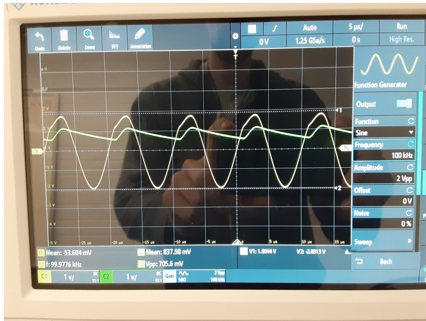
Figure 8. Behaviour of the circuit from Prelab Exercise 10 given a 100 kHz sinusoidal input. v_{in} is yellow and v_{out} is green.
